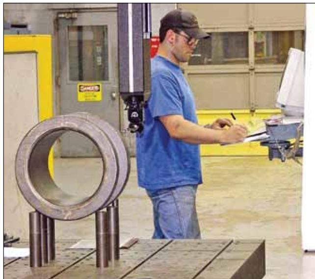
Installing coordinate measuring machines, which verify the dimensional accuracy of castings, is a simple start to performing nondestructive testing.
